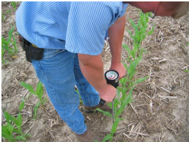
Figure 8. Measuring soil compaction with a soil penetrometer.
