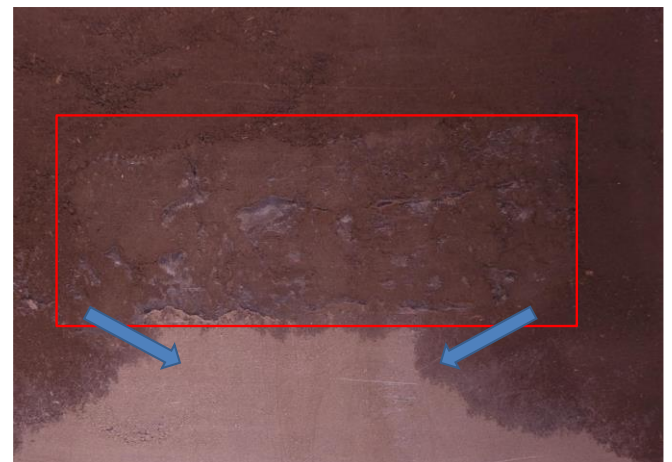
Figure 4. Water, as it drains through the soil profile, is limited by a zone of highly compacted soil (outlined by the red box). Water drains through less compacted soil more quickly and eventually begins to move below the zone of high compaction (Strachan and Jeschke 2017).
